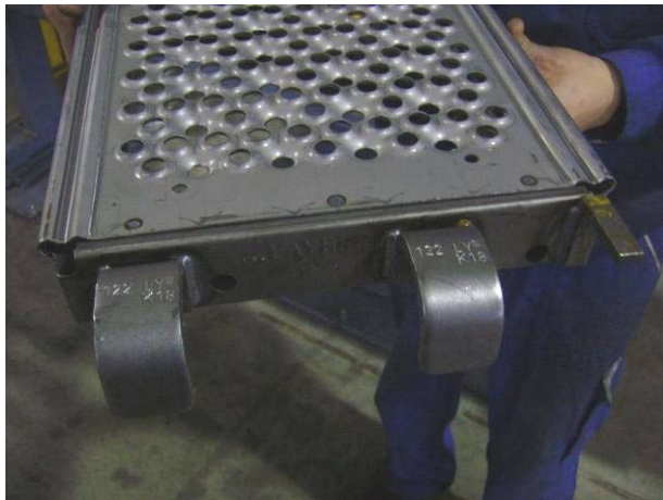
Pic. 2 and 3: Metal board after welding and before zinc coating – NO TOP WELD ON HOOKS!
